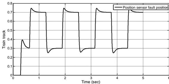
Fig. 11. The trajectory of levitation system in presence of position sensor fault.
