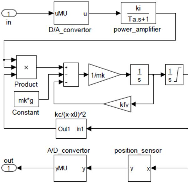
Fig. 3. Simulation scheme of magnetic levitation model.
