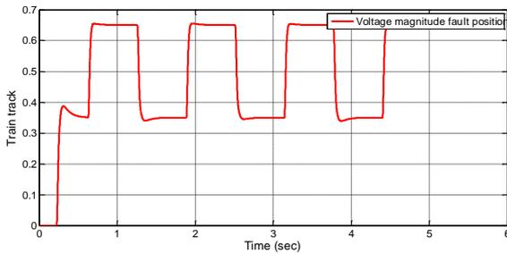
Fig. 10. The trajectory of levitation system in presence of voltage fault.
