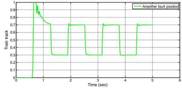
Fig. 12. The trajectory of levitation system in presence of power amplifier fault.
