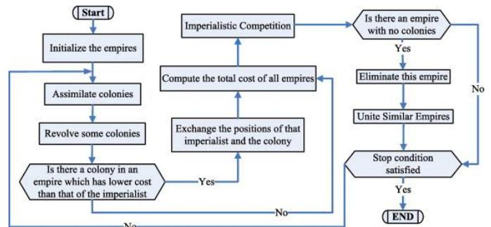
Fig. 7. The main structure of imperialist competitive algorithm.
