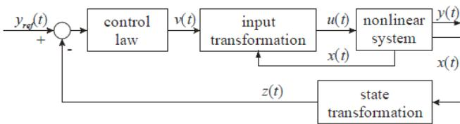
Fig. 5. Control structure using exact feedback linearization method.
