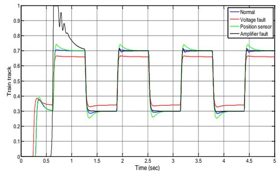
Fig. 13. The trajectory of levitation system in presence of voltage different states.
