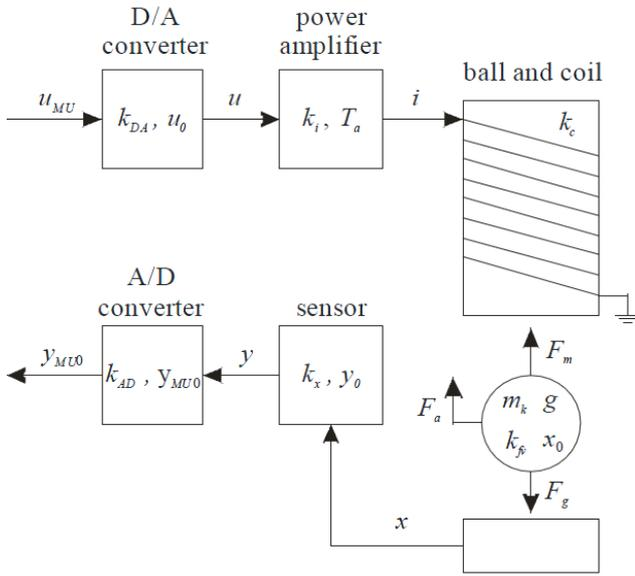
Fig. 2. Magnetic levitation model.
