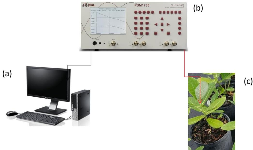
Fig. 2. An illustration to show Electrical Impedance measurements setup (a) Desktop Computer, (b) Impedance Analyzer, (c) *Calotropis Procera* plants
