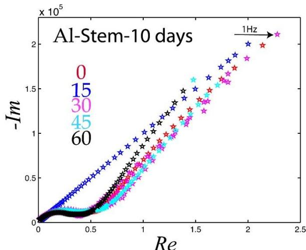
**Fig. 3.** Electrical impedance spectra (EIS) of the stem of *C. procerca* plants cultivated hydroponically under laboratory conditions. The term “Re” refers to the real part ( $Z'$ ) and “-Im” to the imaginary part of impedance ( $Z''$ ). In each curve, the frequency increased from the right (1 Hz) to left (1 MHz). The values are computed following a 10-days treatment with aluminum at different concentrations (0, 15, 30, 45 and 60 mg/l).
