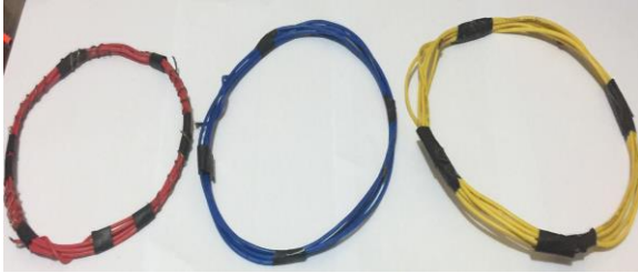
Fig. 2. Coil with 16cm of coil in various type of cores.
