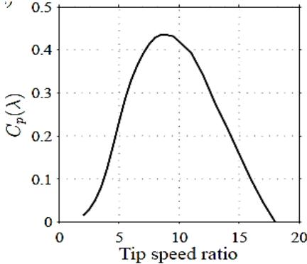
Fig. 2. Power coefficient,  $C_p$  based on  $\lambda$ .
