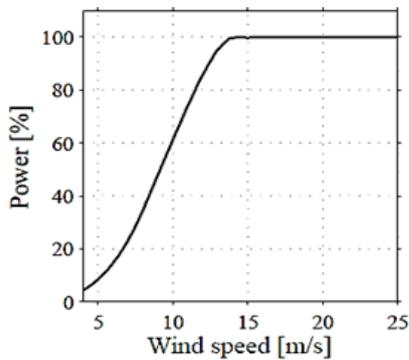
Fig. 3. The power of wind turbine based on wind speed.
