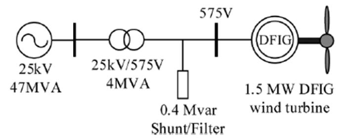
Fig. 9. Linear diagram of studied system.
