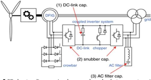
Fig. 5. Wind system diagram using chopper and crowbar (rotor converter-grid converter-crowbar-grid).
