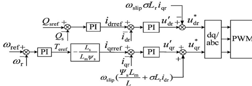
Fig. 6. Control algorithm of rotor in normal mode.
