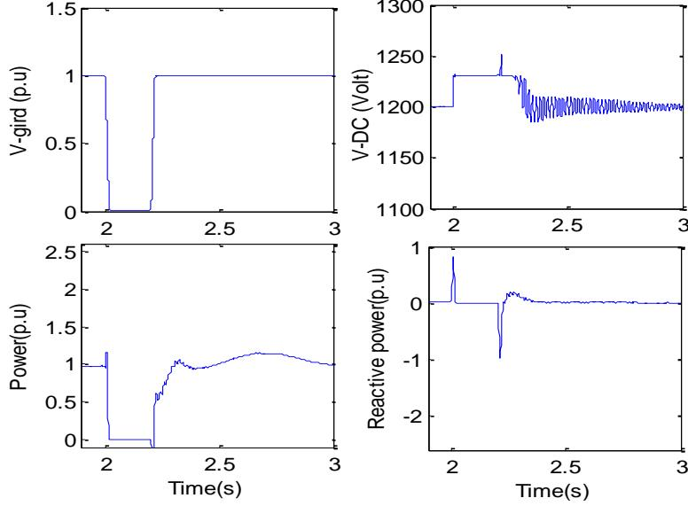
**Fig. 12.** Grid voltage, DC link voltage, active and reactive power (control strategy C).
