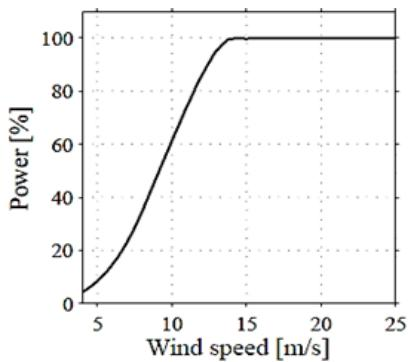
Fig. 3. The power of wind turbine based on wind speed.
