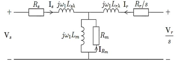
Fig. 4. Equivalent circuit of DFIG.
