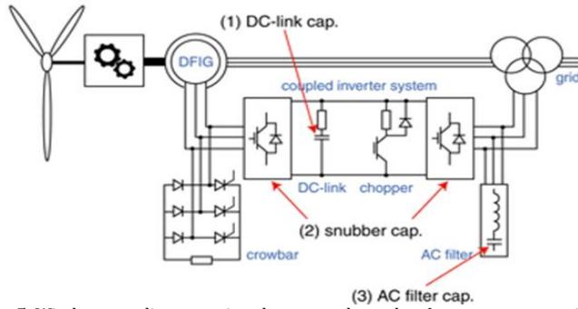
Fig. 5. Wind system diagram using chopper and crowbar (rotor converter-grid converter-crowbar-grid).
