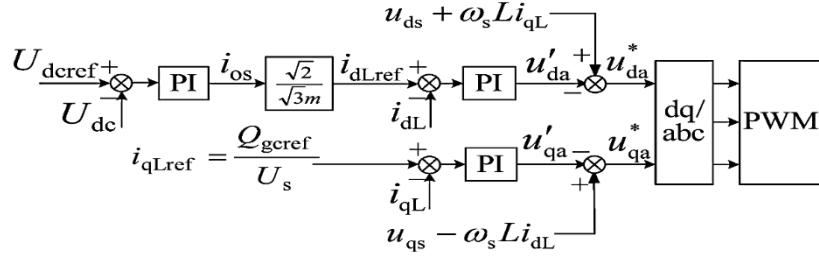
Fig. 7. Control algorithm of grid in normal mode.
