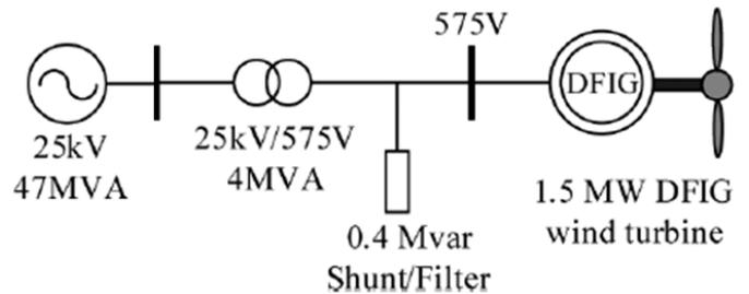
Fig. 9. Linear diagram of studied system.
