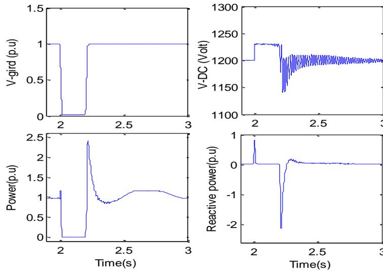
Fig. 10. Grid voltage, DC link voltage, active and reactive power (control strategy A).
