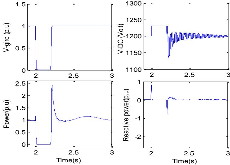
**Fig. 11.** Grid voltage, DC link voltage, active and reactive power (control strategy B).
