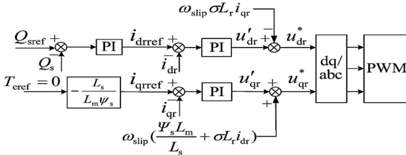
Fig. 8. Control algorithm of rotor in fault mode.
